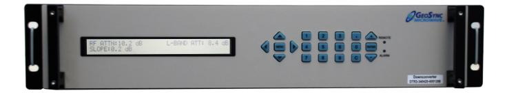
These GeoSync Microwave 2 and 3 Channel Downconverters are designed with shared local oscillators to provide two or three phase and amplitude related channels for tracking applications. Every effort has been made to simultaneously provide high performance, reliability and value. Models are available for operation in either S-, C-, X-, Ku and Ka-Band.
