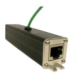
Ventev's Ethernet surge suppressor offers advanced inline, bi-directional lightning and surge protection for Ethernet powered devices. This suppressor is CAT5e/CAT6/CAT6A compatible and includes a single port with shielded RJ45 jacks and metal housing for EMI noise suppression. It is for 802.3bt and is backwards compatible with 802.3at and 802.3af. Every Ventev surge supressor is covered by the company's two-year TerraNet warranty program.
